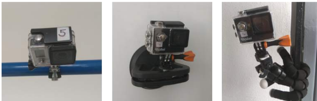
Figure 5.3: Example of mounting solutions of measurement equipment using telescopic building props in combination with pipe clamps ( left ); suction cups ( middle ); flexible tripods ( right )
